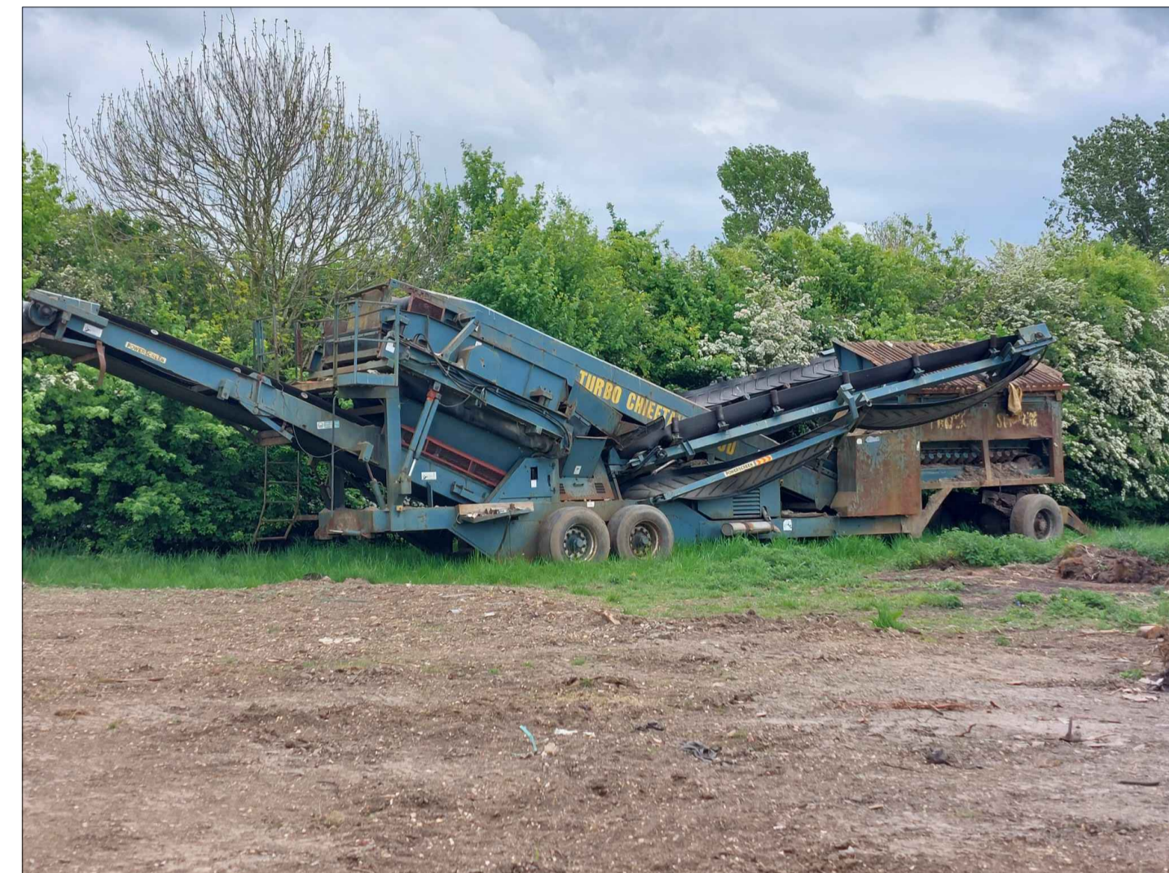
TYPICAL TOPSOIL SCREENER
